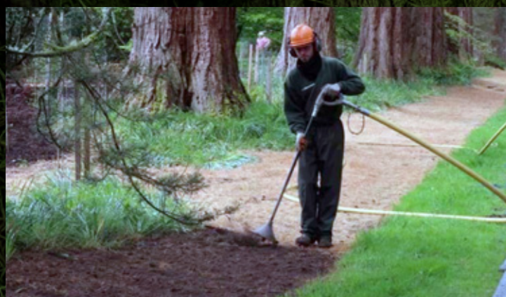
The process involved killing off the grass around the redwoods, then utilising a geo injector to puncture the ground and blow air beneath the surface, breaking-up the compacted soil
